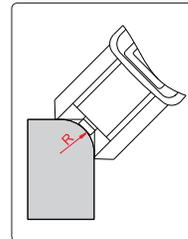
Measure leg length of 45° chamfer
