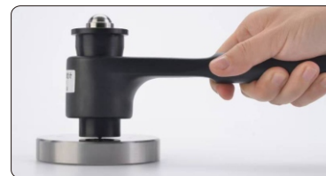
Hammer impact to apply test force
